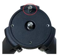
3. <u>Attach mount head</u>: Before put the mount onto the tripod, make sure the RA gear switch is at lock position to prevent mount head free swing by accident! Retract the 2x Azimuth (Azi) Adjustment Screws from both sides to leave ample space for the alignment peg to be fitted in between the 2x Azi Adjustment Screws. Remove the 2x Azi Locking
