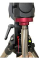
6. <u>Install counterweight</u>: Before putting on CW, make sure the mount is at its zero position, i.e., CW shaft points to the ground. Insert Allen wrench to lock the RA axle and disengage the R.A. Gear Switch to set the R.A. axis free before loading the CW. Remove the CW Safety Cap at the end of CW Shaft. Glide the CW over the shaft with the larger hole opening facing down. Tighten the CW Locking Screw to hold the CW in place. Place the Safety Cap back onto the shaft.
