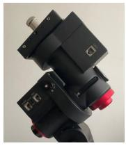
Level the mount by adjusting the tripod legs. Use the build-in Bubble Level Indicator or an external leveler for this purpose.
