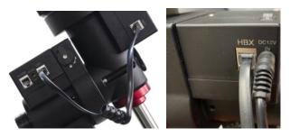
Connect the Go2Nova<sup>®</sup> 8409 Hand Controller to the **HBX** port on the main unit. Plug in a 12V DC power supply to the **DC12V IN** socket next to the **HBX** port.
