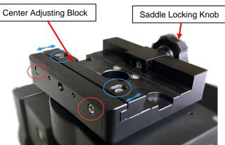
8. <u>Balance payload</u>: After attaching the scope and accessories, the mount head assembly must be balanced in both DEC and RA axes to ensure minimum stresses on the mount driving mechanism.
