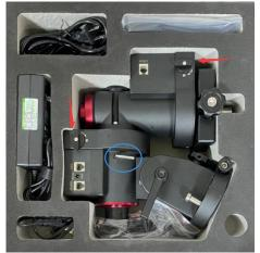
If the mount has a AccuAlign<sup>™</sup> optical pola scope, the Allen wrench may **NOT** be inserted here.
